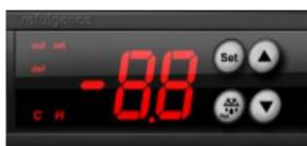
The electronic controller has been factory set to cool the beverages to lowest temperature approximately 1-5 Centigrade. Should you wish to alter the temperature set point, please adopt the following procedure.
